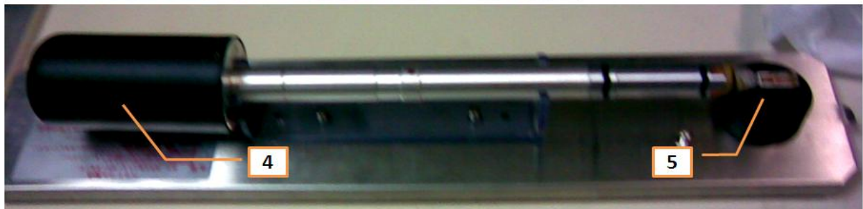
Figure 2 The side entry goniometer stage & specimen holder.
