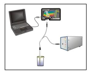
Common transmission applications include measuring light through solutions, optical filters, optical coatings, and other optical elements (such as lenses and fibers).
