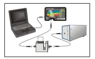
Absorbance is also proportional to the concentration of the substance interacting with the light (this is known as Beer's Law). Common absorption applications include the quantification of chemical concentrations in aqueous or gaseous samples.
