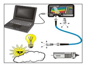
Common applications include characterizing the light output of LEDs, incandescent lamps, and other radiant energy sources such as sunlight. Relative irradiance measurements also include fluorescence measurements, which measure the energy given off by materials excited by light at shorter wavelengths.
