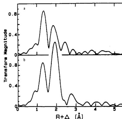
Figure 1. K-edge EXAFS transforms (transform  $k$  range  $4\text{--}15 \text{ \AA}^{-1}$ ): (a)  $[\text{Ph}_4\text{P}][\text{MoOSL}]$  (**1**); (b) *trans*- $\text{MoO}(\text{SH})\text{L}$  (**2**).
