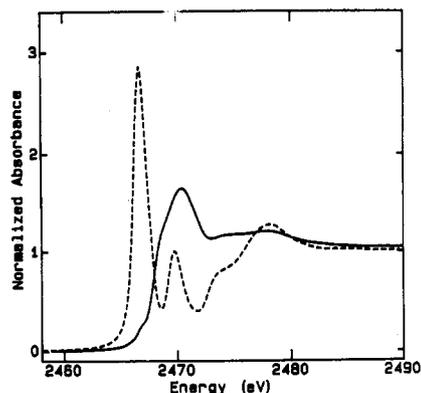
Figure 3. Sulfur K-edge X-ray absorption spectra: (—)  $[\text{Ph}_4\text{P}][\text{MoOSL}]$  (1); (---)  $\text{MoSCl}_2(\text{HB}(\text{Me}_2\text{C}_3\text{N}_2\text{H})_3)$ .<sup>11</sup>
