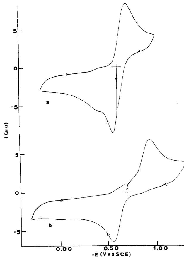
Figure 4. Cyclic voltammograms (in DMF with 0.10 M  $[n\text{-Bu}_4\text{N}][\text{BF}_4]$ , Pt electrode, scan rate  $0.100 \text{ V s}^{-1}$ ): (a)  $[\text{Ph}_4\text{P}][\text{MoOSL}]$  (**1**); (b)  $\text{trans-MoO}(\text{SH})\text{L}$  (**2**).
