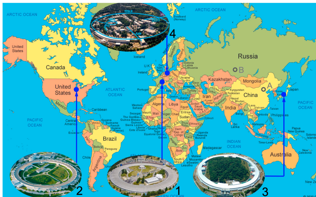
Figure 3. Synchrotron radiation facilities around the world which have nuclear resonant scattering (NRS) beamlines (solid blue symbols): 1 = ESRF, with 6 GeV electron energy and 0.9 km circumference, operating since 1994; 2 = APS, with 7 GeV electron energy and 1.1 km circumference, operating since 1995; 3 = SPring-8, with 8 GeV electron energy and 1.5 km circumference, operating since 1996; 4 = Petra-III, with 6 GeV electron energy and 2.3 km circumference, operating since 2009. The gray circles indicate the possible NRVS-suitable rings in the future: A = HEPs, with 6 GeV electron energy and 1.4 km circumference; SKIF, with 3 GeV electron energy and 0.5 km circumference.
