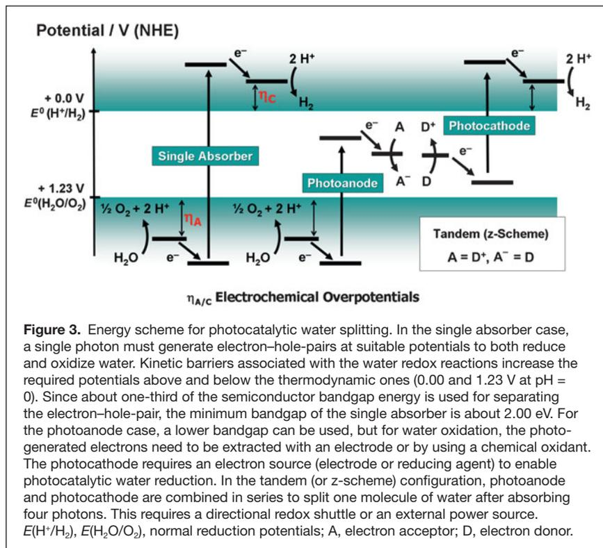
the quantum yield is reduced by a factor of two, because now two photons are required to generate one electron–hole-pair of sufficient energy to split water. The result is that considerable higher efficiencies can be achieved in these multijunction devices. For a tandem device with two bandgaps of about 1.9 and 1.2 eV, a maximum practical water splitting efficiency of about 15% can be achieved. More detailed treatments of these efficiency limits are given in the literature.<sup>12–14</sup>
